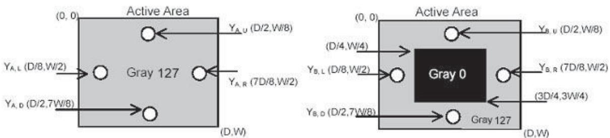
**Note 9: Test Pattern: Subchecker Pattern measured by TOPCON SB**
