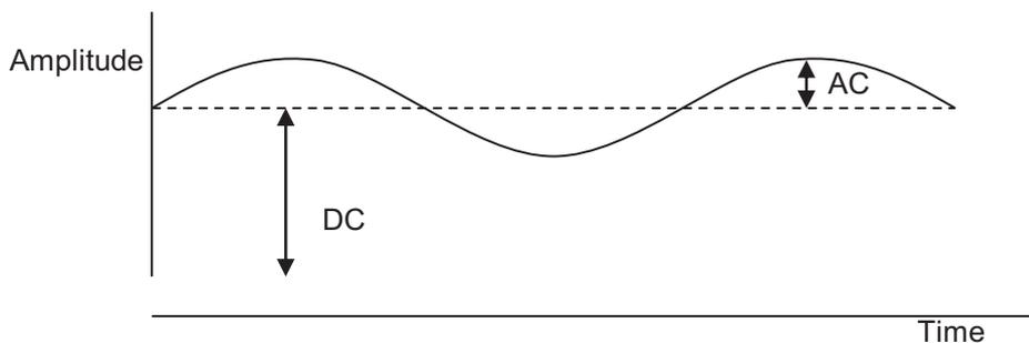
$$\text{Flicker (dB)} \square 20 \log \frac{\text{AC Level (at 30Hz)}}{\text{DC Level}}$$
